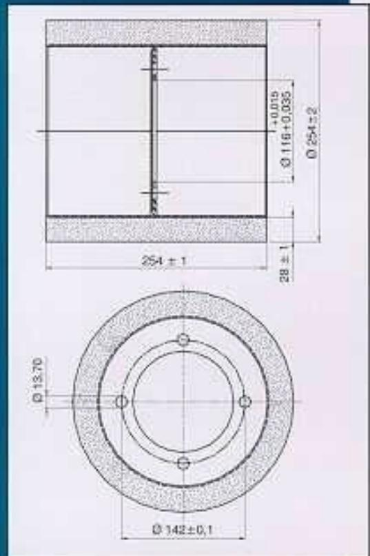
The metal nucleus of the Zaccaria 10''x10'' rubber rolls, which is also produced by Zaccaria, is made of steel sheet. It is submitted to a special surface treatment, being that the world's best adhesives are applied on them for proper adhesion between the two parts.
